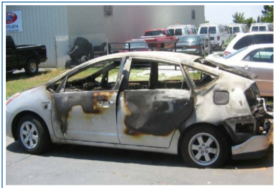
FIG. 2. Full vehicle loss from battery pack thermal runaway in an aftermarket modified vehicle.
